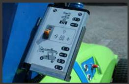
Multifunction control panel in operator friendly design with integrated push buttons and signal lights. Full monitoring of machine capacity limits for increased security.
